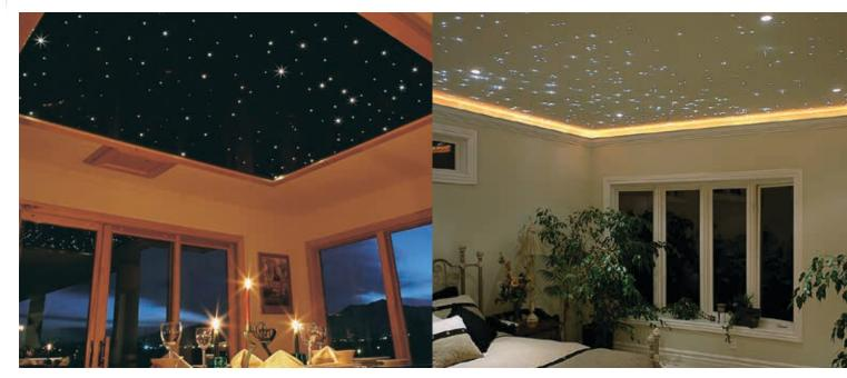
Galaxy Fiber Optic Systems are comprised of a fiber optic illuminator with a LED or Halogen light source, 12' long, 1.0mm dia. clear acrylic fibers, and acrylic panels or existing ceiling/wall covering drilled to accept the fibers. Fiber optic illuminators ship with a black/white wheel for a twinkling star night effect, and a color wheel for a kaleidoscope effect. Standard acrylic panels fit into a 2' x 2' or 2' x 4' drop ceiling. Custom panel sizes are available, up to a maximum 4' x 8' panel.
