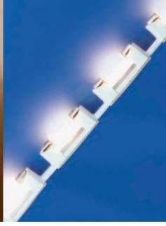
With a bend radius of 2.25" (5.75cm), inside or outside, Xenon Brightstrip can evenly illuminate the tightest of curved surfaces. Even 90 degree corners are simple to do. Xenon Brightstrip mounts easily with 3M® double sided tape (pre-fixed to the back of each socket) or with simple to use nail clips for added security. The lamp holders have a metal reflector built in which deflects heat away from the mounting surface and reflects light onto the surface being illuminated.
